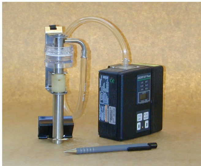
Figure 2-1. Gravimetric sampling pump, cyclone and filter cassette.
